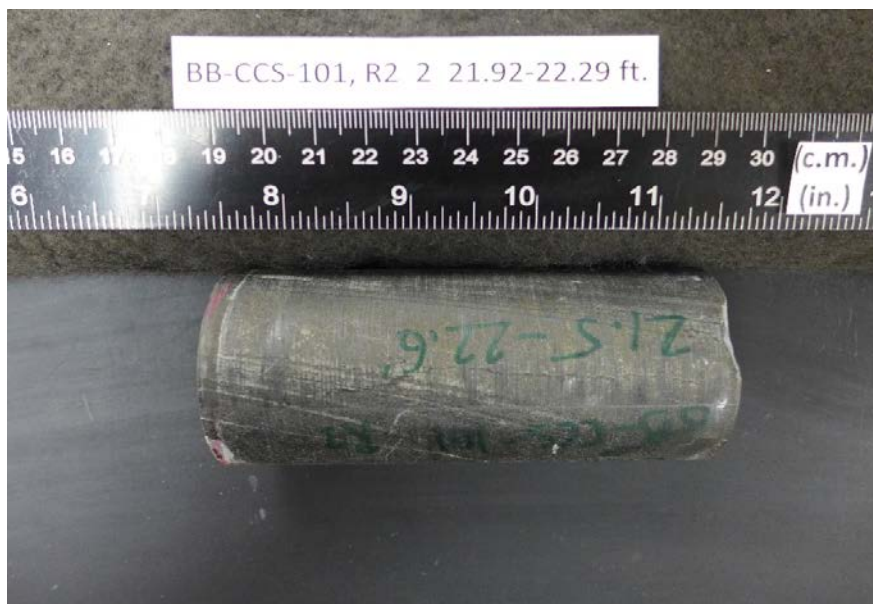
After cutting and grinding
