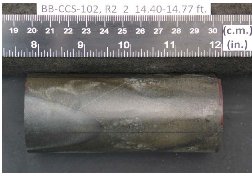
After cutting and grinding
